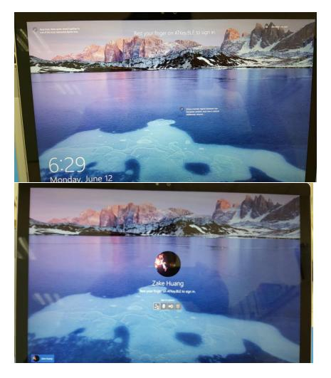
Limitation from Windows 10: CDF device can't logon at cold boot or Windows reboot since it needs password or PIN code by design; but from Windows 10 build 1709 (RS3), it can support CDF login even at cold boot or reboot.
