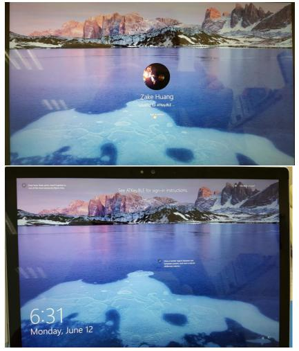
Message showing on screen: "Rest your finger on ATKey.BLE to sign in", and LED is flashing Blue, please put your fingerprint on, till Green LED shows (or Red); then it will auto-unlock to Windows.
