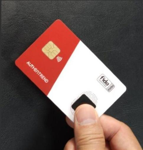
Take the card by “enrolled” thumb finger (on fingerprint sensor sear) and index finger (on back)
